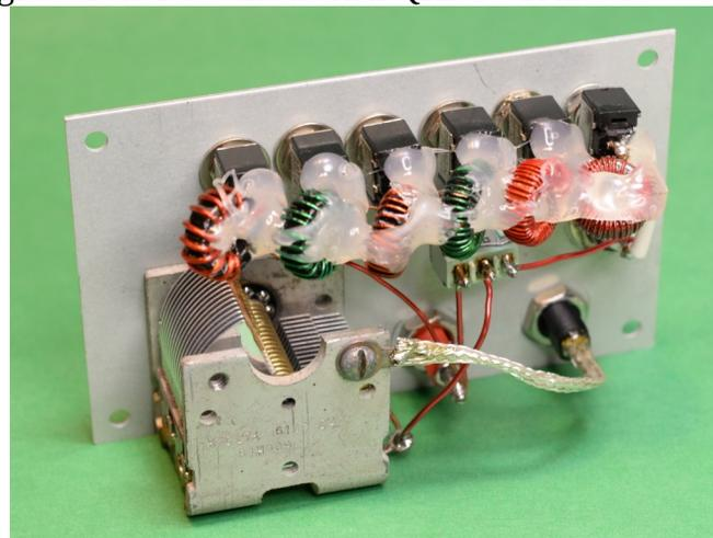
Front and back of the Tuner. This version has an extra 8μH inductor, that has never been needed, and is used with an external SWR metering circuit. The variable capacitor is a 30pF to 440pF unit.
